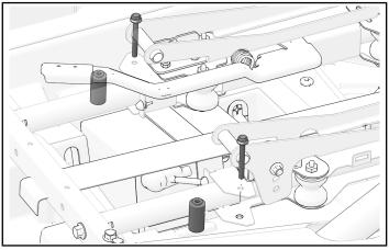
3. Stack harness brackets atop each spacer groove.
