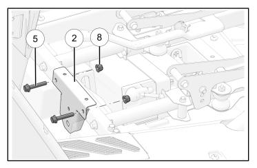
2. Mount retractor/harness assembly ① onto retractor bracket ② with one nut ⑧.
