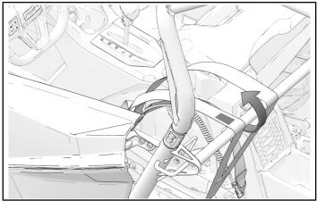
2. Remove and retain two bolts and two spacers from seat roller brackets.
