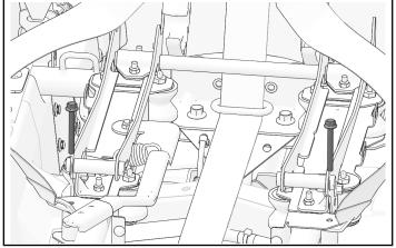
5. Install rear harness brackets onto rear seat base with one harness fastener (7) and one nut (8) per side.
