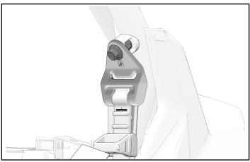
4. Remove and discard one nut from seat belt retractor.
