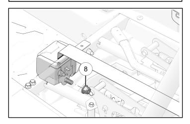
Install front harness guide ③ onto retractor bracket
