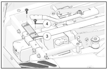
4. Mount rear harness guide onto stud with one nut
