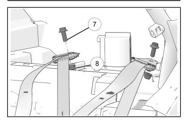
Multi-Passenger Models: Extend harness behind-and-over harness bar.
