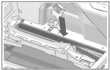
6. Remove and discard bolt <sup>©</sup>. Remove and discard seat belt buckle.
