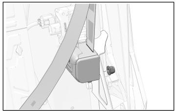
4. Remove and discard nut <sup>®</sup> from buckle connecting bolt. Disconnect speed-regulator connector. Remove and discard seat belt buckle.
