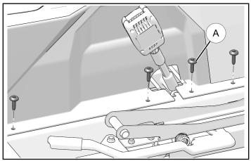
2. Remove and retain four screws (A) from RH center console panel.
