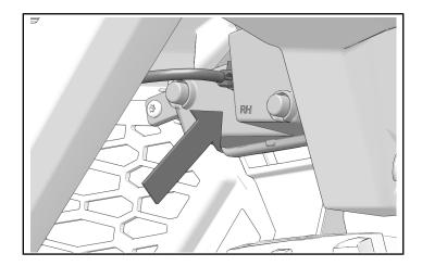
5. Remove and keep four push pin rivets.
