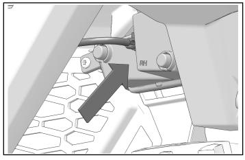
5. Position front bumper ① and loosely install two upper screws ④.
