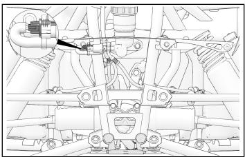
8. Remove and discard two screws from front fascia bracket. Remove and discard front fascia bracket.
