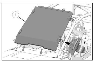
2. Close Lock & Ride® clamps ④ to secure windshield to ROPS.
