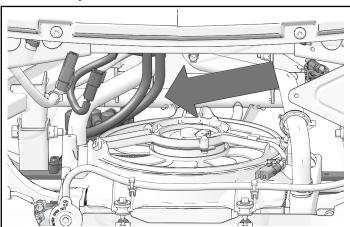
5. Route winch power wires under frame assembly, then up behind PULSE® board. Install push pin clips into frame as shown.
