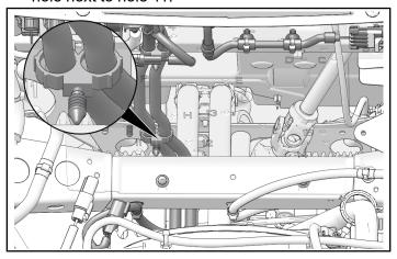
7. Route wires through opening in PULSE® board.
