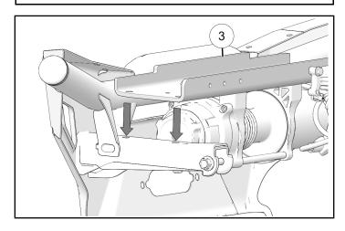
2. Install screws (9) into mounting plate (6). Make sure winch assembly (3) sits flush on bumper. Torque to specification.
