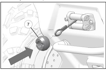
2. Install winch hook ® onto winch cable using pin A and hairpin clip. Bend ends of clip around pin to secure.
