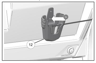
3. Install remote control mount ① using two screws ④.
