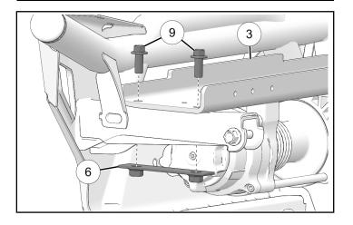
3. Install bumper on vehicle using kept screws and nuts (upper nut ® not shown). Torque to specification.
