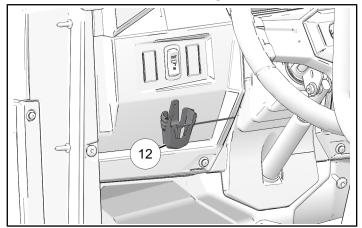
2. Locate and drill two holes. Use remote control mount ① as a template to mark the holes.
