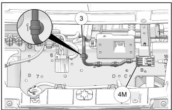
2. Install harness in clip located behind PULSE® bar. Route inside vehicle along existing wiring and connect **4F** to vehicle accessory power.
