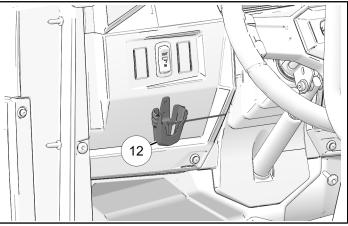
2. Locate and drill two holes. Use remote control mount 1 as a template to mark the holes.
