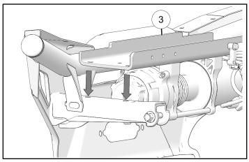
2. Install screws (9) into mounting plate (6). Make sure winch assembly (3) sits flush on bumper. Torque to specification.
