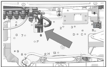
8. Connect the winch power wire (A) and winch ground wire (B) to PULSE® bar as shown. Torque to specification.
