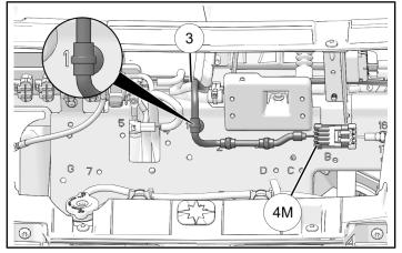
2. Install harness in clip located behind PULSE<sup>®</sup> bar. Route inside vehicle along existing wiring and connect **4F** to vehicle accessory power.
