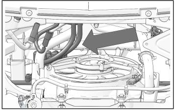
5. Route winch power wires under frame assembly, then up behind PULSE<sup>®</sup> board. Install push pin clips into frame as shown.
