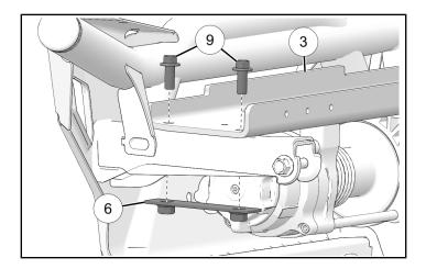
3. Install bumper on vehicle using kept screws and nuts (upper nut <sup>®</sup> not shown). Torque to specification.
