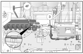
3. Route wiring along rear of compartment. Secure in positions shown. Route inside vehicle along existing wiring and connect **12F** to winch switch.
