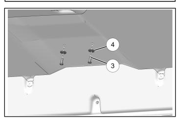
11. Install middle of rear roof liner to roof with two screws ③ and two washers ④. Torque screws to specification.
