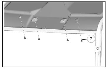
9. Install rear of roof liner to roll cage with two pushdarts  $\widehat{\mathcal{T}}.$
