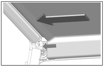
7. Make sure both sides of rear liner are placed between roof and roll cage.
