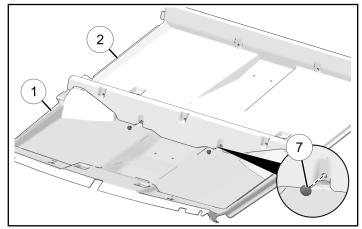
3. Put roof liner assembly in vehicle, through passenger side, and align with roof.
