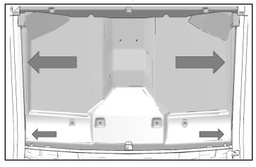
6. Put tabs of rear roof liner between roof and roll cage.
