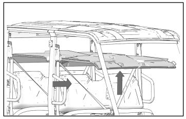
4. Put tabs of front roof liner between roof and roll cage.
