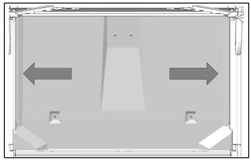
8. Install front of roof liner to windshield mounting plate with four push-darts  $\overline{O}$ .
