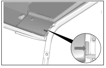
5. Make sure both sides of front roof liner are placed between roof and roll cage.
