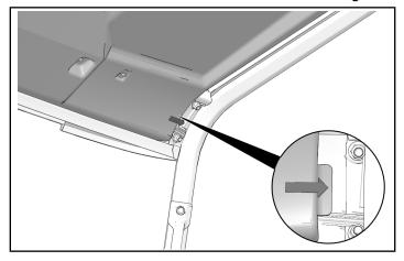
3. Make sure both sides of roof liner are placed between roof and roll cage.
