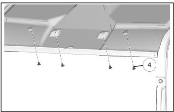
5. Install rear of roof liner to roll cage with two push-darts (4).
