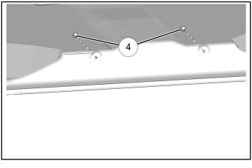
6. Install middle of roof liner to roof with two screws
