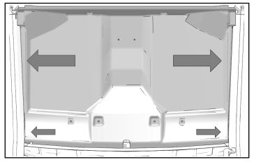
4. Install front of roof liner to windshield mounting plate with four push-darts ④.
