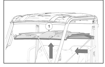
2. Put tabs of roof liner between roof and roll cage.
