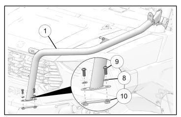
Loosely install left hood rack bar ① to left ROPS clamp ⑤ with two washers ⑧ and two screws ⑨. Repeat for right side.
