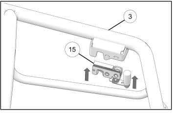
4. Loosely install each latch assembly to the hood rack basket ③ with two screws ⑧, two washers ⑲, and two nuts ⑳.
