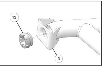
2. Install seat latch pin 1 into each grommet 1.
