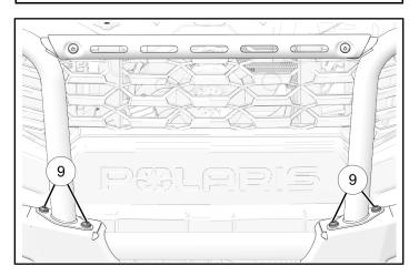
2. Counter hold nuts (1) and torque front upper bumper tube screws (9) to specification.
