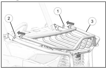
4. Loosely install the hood rack basket nuts (1) to each hood rack basket latch pin (1).
