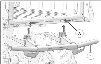
2. Loosely install rear bumper ① to chassis bar with screws ④ and nuts ⑤.
