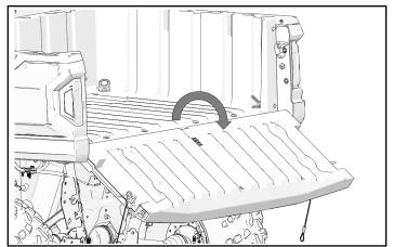
3. Pull left side of tailgate down, then move tailgate off of right side pivot on cargo box.
