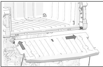
2. Attach cables to screws on cargo box.
