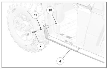
8. Install the rear portion of the rock slider 4 to the rear bracket with the screws 8 and washers 11.
