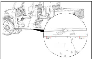
6. Install the L-shaped weld nut brackets ① into the slot and onto the frame of the vehicle.
