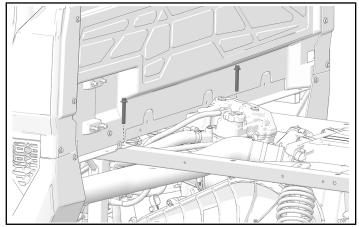
2. Use the retained bolt and nut to install the back bracket ② of the rock slider to the box frame.
