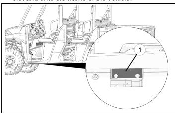
7. Hold the rock slider ④ in place. Install the front bolt ①, washer ⑪, and nut ⑩
