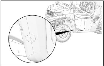
5. Cut the tabs off the skid plate to allow clearance for the lower bolts.
