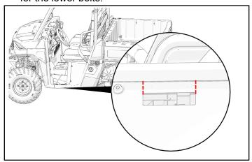
6. Install the L-shaped weld nut bracket ① into the slot and onto the frame of the vehicle.
