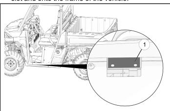
7. Hold the rock slider ④ in place. Install the front bolt ①, washer ⑪, and nut ⑩
