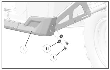
9. Install the screws (9) into the bottom of the rock slider, through the frame of the vehicle and into the L-shaped backer plate.
