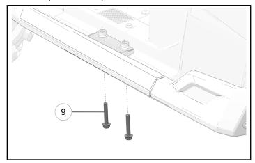
10. Torque all fasteners to specification.
