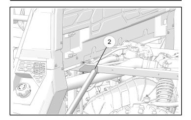
3. Install the lower piece of the back bracket with the bolt  $\widehat{\mathcal{D}}$ .
