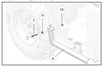
8. Install the rear portion of the rock slider 4 to the rear bracket with the screws 8 and washers 11.
