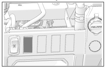
20. Install switch ① to switch connector 12F.
