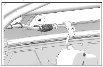
26. Install washer hose ③ and secure with cable tie.
