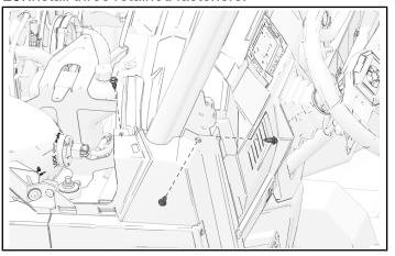
24. Peel backing from routing channel ⑨ and install on ROPS.
