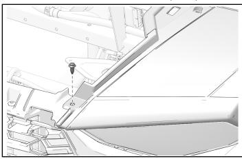
32. Install rear of outer hood with one retained screw.
