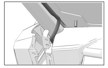
23. Install three retained fasteners.
