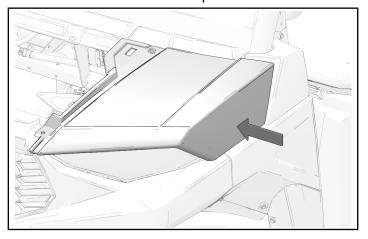
31. Install front of outer hood with one push-pin rivet.
