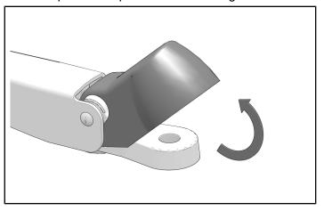
12. Put wiper arm on to wiper arm shaft in a position that will allow wiper blade to fully clean windshield.
