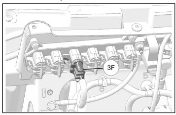
18. Install fuses to electrical mounting panel.
