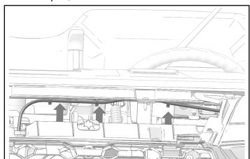
28. Drill a 5/16 in (8 mm) hole 6 1/4 in (16 cm) away from inner edge.
