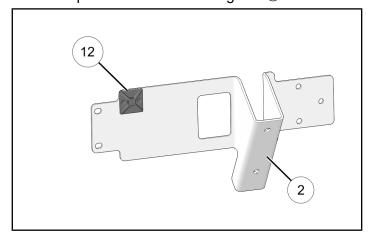
2. Install washer fluid reservoir bracket ② using screws ⑭.
