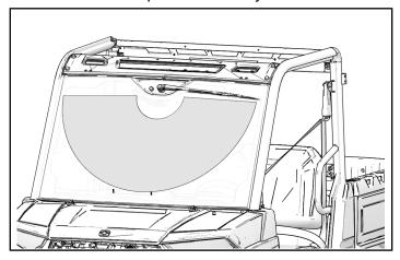
13. Install wiper using washer 3 and nut 2.
