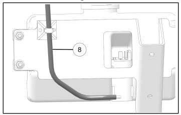
27. Attach washer hose to bottom of upper dash panel with clips 10.
