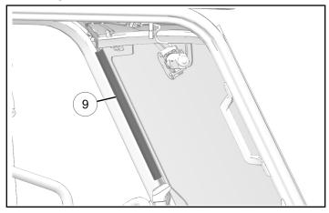
25. Attach harness to ROPS using clips and connect **4F** to wiper motor.
