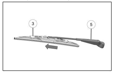
11. Lift wiper arm cap to reveal mounting bracket.
