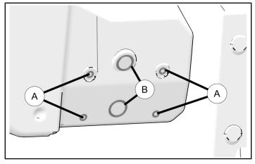
7. Drill two 1 inch holes (B) for the heater hoses.
