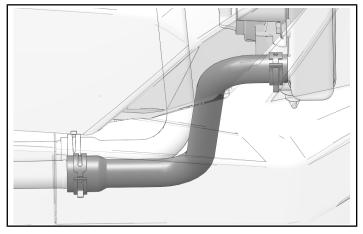
29. Assemble coolant hose (5), radiator hose (6), tee connector (6) and spring clamps (2) and (2) as shown.
