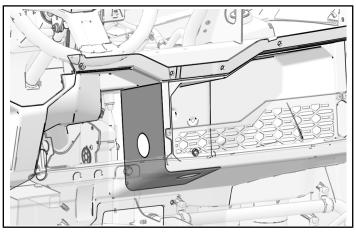
11. Using 2 inch hole saw, drill holes. Deburr the holes to remove rough edge.
