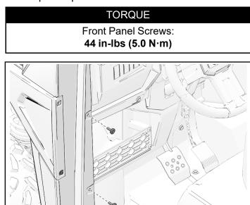
5. Torque two upper dash screws to specification.
