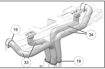
Install longer air ducts 3 on the driver's side air vents and heater assembly. Secure with cable ties
