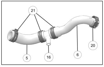
30. Install the hose assembly to the radiator and the coolant hose as shown.
