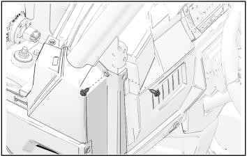
4. Install front frame panel with two retained screws. Torque to specification.
