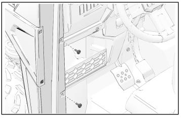
2. Remove and keep two push-pin rivets from front frame panel.
