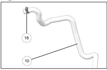
39. Install the hose assembly onto the thermostat housing. Tighten hose clamp (18) to specification.
