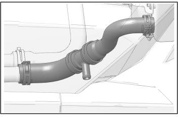
31. Install heater hose (1) to tee connector (6).
