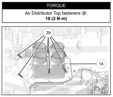
15. Install heater control panel ④. Torque fasteners <sup>(29)</sup> to specification.
