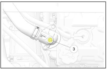
7. Fill the radiator until a steady stream of coolant begins to drain out of the bleed screw.
