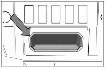
3. Remove and keep four screws from dash compartment cover.
