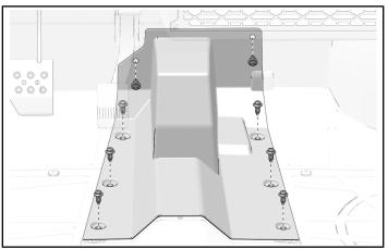
2. Remove tunnel cover from vehicle.
