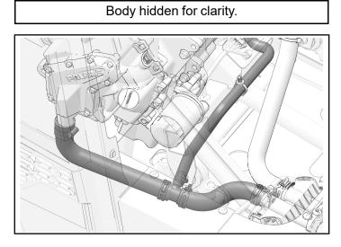
37. Install new engine inlet hose (8). Secure with new worm clamp (2) and spring clamp (2).
