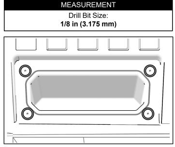
2. Score storage compartment in the main dash and cut out for heater control panel.
