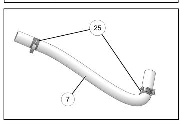
26. Install onto heater assembly. Do not clamp hose fitting at this time.
