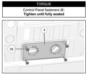
16. Route control panel harness (2) through bulkhead and connect to control panel and heater assembly.
