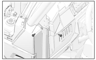
3. Remove and keep four push-pin rivets from upper dash.
