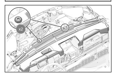
2. Install upper dash with four retained push-pin rivets, as shown.
