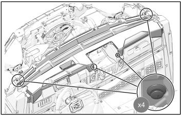
3. Install front frame panel with two retained push-pin rivets.
