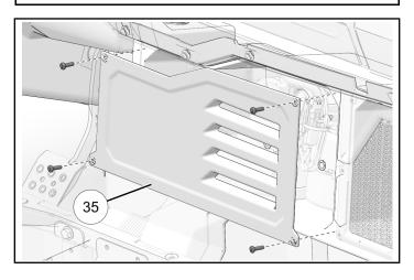
5. Install two new screws (2) into upper dash to fill the void left from the previous net screws, as shown. Torque to specification.
