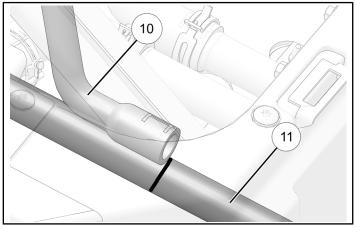
41. Cut the coolant hose all the way through at the mark.
