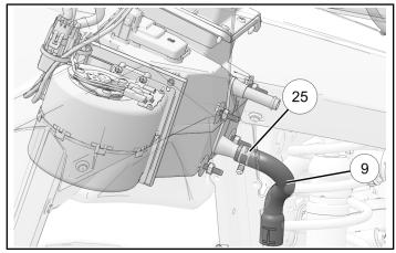
23. Install spring clamp <sup>(2)</sup>, straight connector <sup>(7)</sup>, tree clip <sup>(2)</sup>, hose clamp <sup>(2)</sup> and long heater hose <sup>(1)</sup> to the front heater hose <sup>(9)</sup> installed in the previous step. Torque hose clamp to specification.
