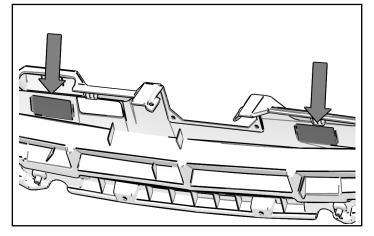
2. Drill 1/8 inch pilot hole through back of upper dash at scribe mark. Then, drill 2 ½ inch hole through the front of the upper dash.
