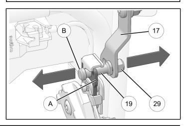
b. HEIGHT: Pin <sup>(1)</sup> should be centered vertically in opening of latch pawls <sup>(A)</sup>. To adjust, loosen two screws <sup>(3)</sup>, slide striker bracket <sup>(7)</sup> up or down as required, then retighten screws.
