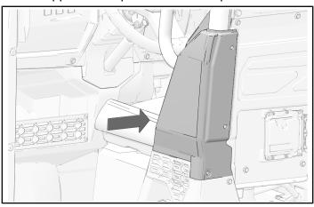
2. Rotate hook over bolster tube.
