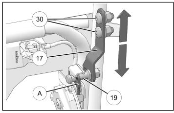
c. **DEPTH**: As required to achieve desired fairing between door frame ① and ROPS/chassis door structure. To adjust, loosen the striker <sup>(1)</sup> and nut <sup>(2)</sup>. Slide striker <sup>(1)</sup> inboard or outboard on the striker bracket as required, then reinstall striker and nut.
