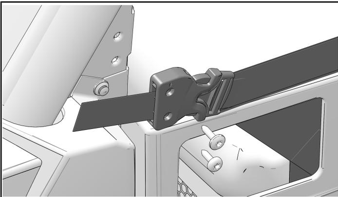
3. Remove and retain the lower side net fastener on the floorboard. Continue by reinstalling the retained lower fastener and torquing to specification.
