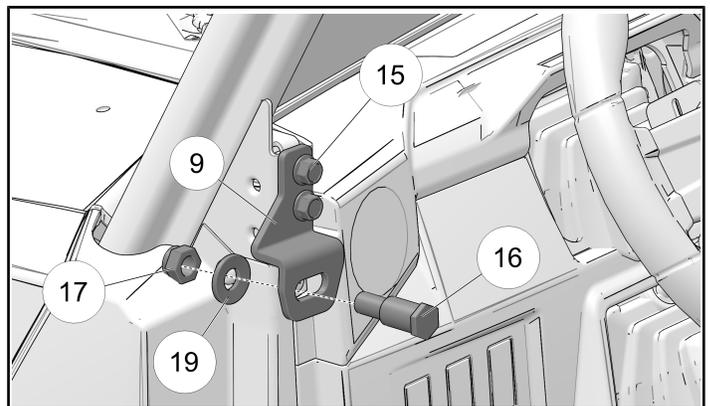
18. Lift the door up and over the adjustment tool and slowly close the door to observe the striker pin ⑯ entering the latch assembly. Ensure the door double latches and adjust the position as necessary.
