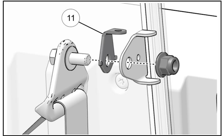
28. Next, install a fastener **14** and spacer **7** into the top of the limiter strap post mount **11** and secure with a nut **18**. Align the hole in the limiter strap with the limiter strap post and press the strap down around the post. Continue by torquing the fastener to specification.
