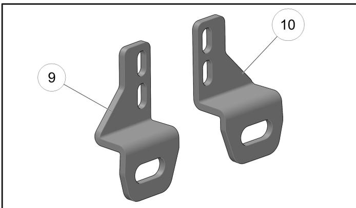
16. Loosely align the striker mount ⑨ with the mounting holes on the ROPS and install two new fasteners ⑮.
