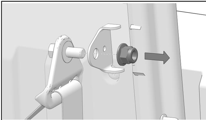
27. Insert the fastener through the seat belt mounting point, washer and the limiter strap post mount **11** with the tab up and facing inward. Continue by inserting the assembly into the ROPS bracket and reinstall the nut. Torque the nut to specification.
