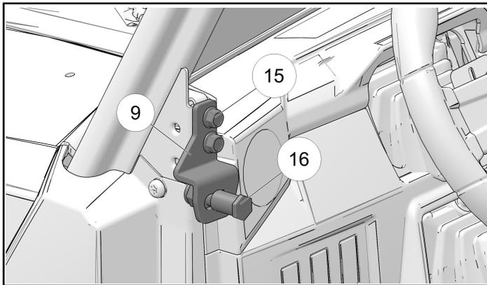
24. If you are unable to achieve proper adjustment, the lower bracket can also be adjusted inwards or outwards by removing the side bezel and loosening the mounting fasteners.
