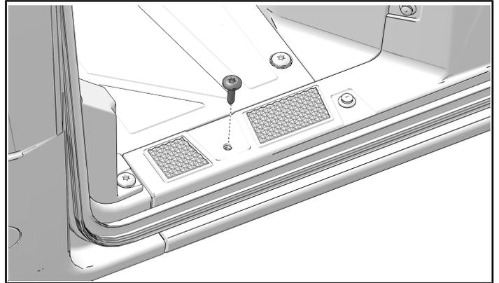
4. Remove and retain the fastener from the lower floor trim piece and remove the two push-pin rivets from the trim piece. Remove the trim.
