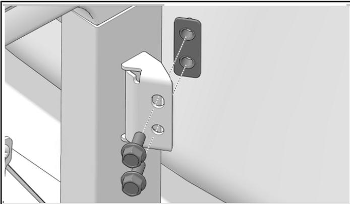
2. Remove the fasteners from the side net latch on the ROPS and remove the latch.
