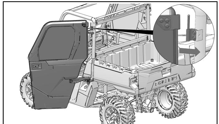
13. Press shim door adjustment tool ⑬ onto the lower door frame.
