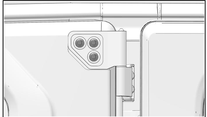
21. Torque the lower door hinge fasteners to specification.
