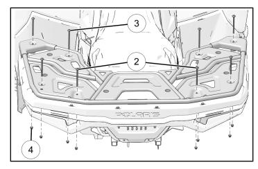
3. Counter-hold nuts and torque all screws to specification.
