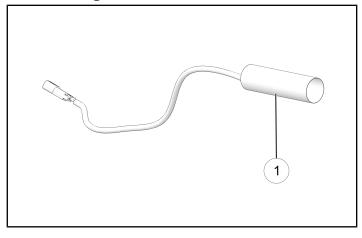
4. Install the hand warmer ① around the right side of the handlebar.
