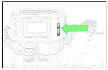
13. Install the thumb warmer switch ⑤ and hand warmer switch ⑥ through the front side of the rear pod.
