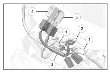
16. Plug the wire harness connector labeled P1 and P2 into the main wire harness. You do not need to plug anything into the other wire harness connector labeled P1 and P2. See page 2 for more information.
