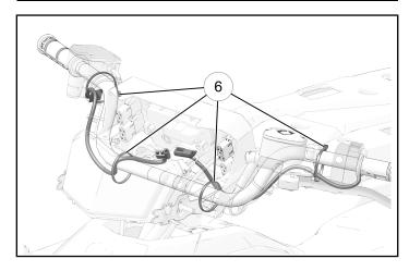
15. Install the wire harness ③ provided with the kit. The wire harness is labeled for each connection. See page 2 for more information.
