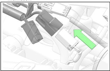
17. Install the front half of the pod and the four headlight pod screws. Torque screws to specification.
