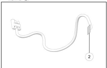
6. Install the thumb warmer ② onto the front of the throttle control lever.
