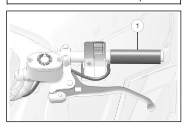
9. Install each handlebar grip back onto the handlebar.
