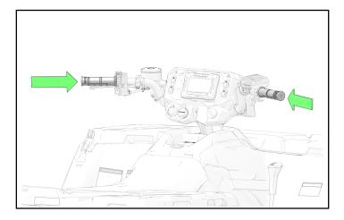
2. Use a solvent wipe to clean the right side of the handlebar and the throttle control lever.
