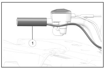
5. Remove the adhesive backing on the thumb warmer ②.
