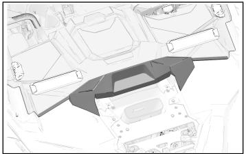
3. With windshield in correct position, lock Lock & Ride<sup>®</sup> clamps around roll-cage.
