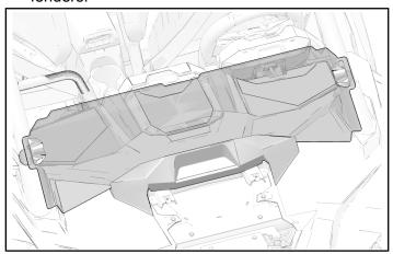
3. With windshield in correct position, secure to ROPS with two Lock & Ride® clamps.
