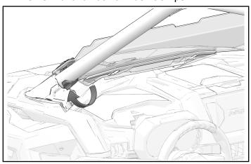
4. Windshield may need repositioning. If needed, release clamps and move windshield upwards along roll-cage.
