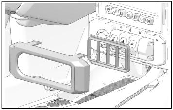
2. Put display center in place and install retained fasteners.
