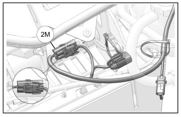
6. Attach fuse holder and vehicle power connection to vehicle as shown.
