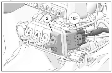
4. Route accessory power harness ③ along existing wiring through firewall and under coolant overflow reservoir as shown. Attach with cable ties ③ at white tape marks.
