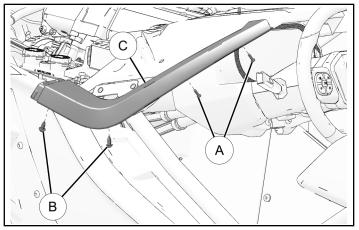
2. Torque two screws to specification.
