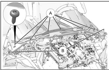
3. Torque eight screws to specification.
