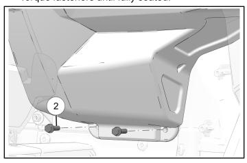
4. Torque two top fasteners to specification.
