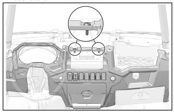
3. Reach through opening and remove one fastener, connecting the bracket to the cross-beam.
