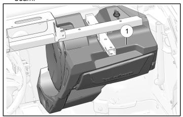
2. Install subwoofer to cross-beam with two retained storage bin fasteners.
