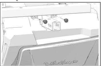
3. Install subwoofer with two accessory fasteners ②. Torque fasteners until fully seated.
