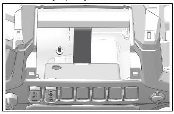
3. Torque three front dashboard fasteners to specification.
