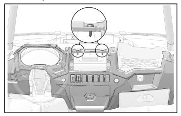
2. Reach through opening and install one fastener.
