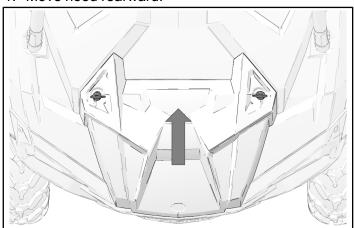
2. Turn quarter-turn fasteners to lock hood to vehicle.
