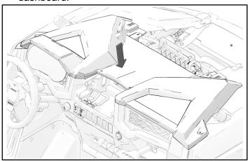
2. Install dashboard with four dashboard fasteners.
