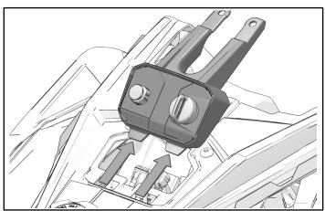
5. Locate witness mark at center of console switch area. Using a drill and 5/32 in drill bit, drill around the witness mark.
