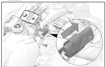
Connect the main harness connector 1A of the heated seat jumper harness to the driver seat heater switch connector of the main harness. Attach wiring to chassis with cable tie.
