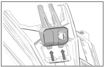
5. Locate the switch witness mark on the back side of the bezel. Using a drill and 5/32 in drill bit, drill around the witness mark.
