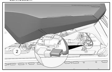
3. Turn latch at rear of seat to lock seat onto snowmobile.
