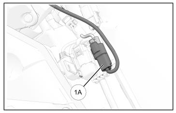
3. Route the heated seat jumper harness ① upward and align the retention location tape of the jumper harness with the retention location of the main harness. Secure the heated seat jumper harness to the main harness with the provided cable tie ④.
