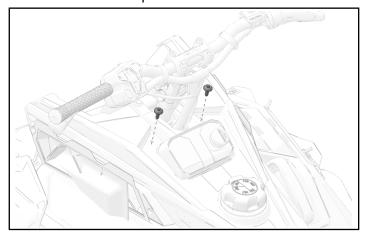
3. Remove and keep two screws and one push pin rivet.
