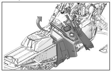
2. Install fuel cap and fuel tank retainer nut.
