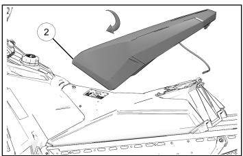
2. Connect heated seat ② plug to chassis connection.
