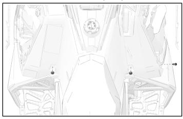
6. Install secondary clutch tool.
