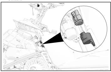
2. Connect the main harness connector **1A** of the heated seat jumper harness to the driver seat heater switch connector of the main harness.
