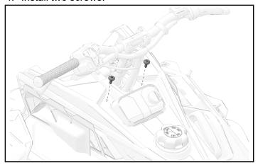
5. Install two screws and one push pin rivet.
