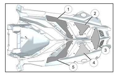
Push foam panel with hands to attach. Start with strokes in the center of foam piece and move from center to edges.
