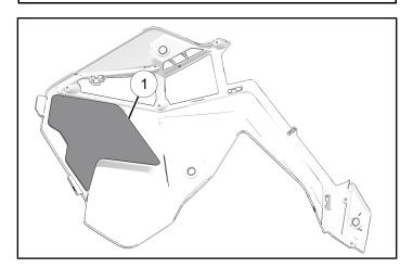
3. Push foam panel with hands to attach. Start with strokes in the center of foam piece and move from center to edges.
