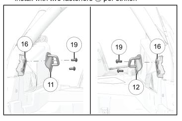
2. Tighten fasteners enough to allow striker to move up and down.
