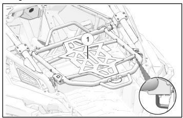
2. Install pivot pins ® through bracket, spacer ②, and into tire rack.
