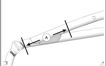
2. Install pivot clamp assembly with top clamp (5) and four fasteners (8).
