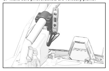
6. Make sure pivot clamp assemblies are correctly spaced apart, according to measurement below. Measure from pivot pin hole to pivot pin hole.
