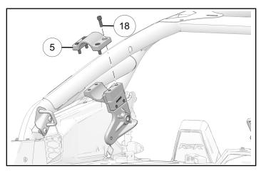
3. Verify pivot bracket fasteners are at the same torque specification. Re-torque if needed.
