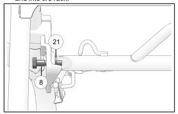
3. Tighten pivot bracket clamp fasteners ® to specification.
