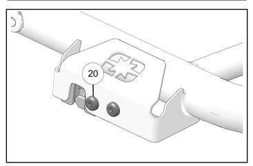
9. Install each strut (4) onto tire rack and pivot bracket.
