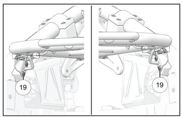
8. Torque latch fasteners ② to specification.
