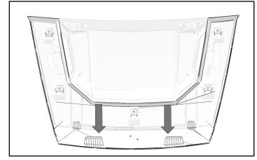
2. Using a cutting tool to trim areas as marked below.
