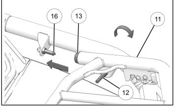
10. Adjust hood rack as necessary until it fits securely.
