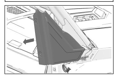
3. Find and mark two drilling point dimples on a-pillar panel.
