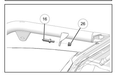
8. Loosely install latch pin <sup>(1)</sup> to hood rack assembly using one nut <sup>(2)</sup>.
