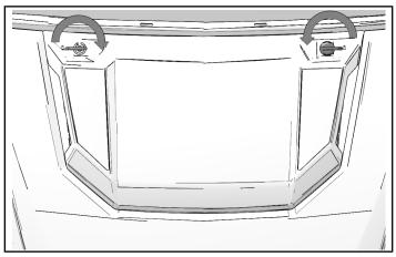
2. Remove hood forward to release front hooks.
