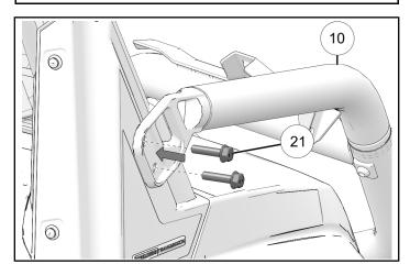
4. Torque two a-pillar screws 1 to specification.
