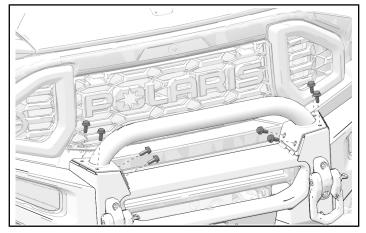
2. Loosely attach middle bumper ③ to mounting point on the vehicle using six screws ⑦.
