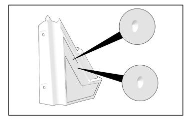
4. Drill two previously marked drilling points on a-pillar panel.
