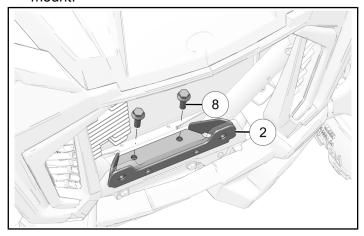
3. Pass nut-plate (§) through front suspension mount and align with fasteners installed in previous step.
