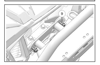
12. Secure lower bumper with two fasteners **3**.
