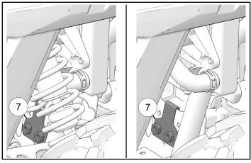
8. Make sure backer plate is aligned with holes in bumper support.
