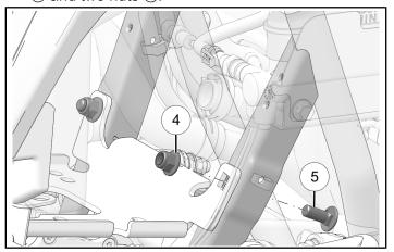
3. Install front of winch mount with two carriage bolts5 and two nuts 4.
