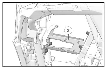
1. Install winch mount ③ on chassis, between front suspension.
