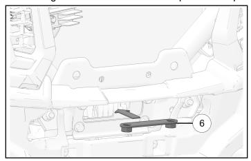
4. Thread two fasteners ® into weld nuts 6.
