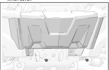
2. Place support bracket ② onto front suspension mount. Pass two fasteners ⑧ through bracket and mount.
