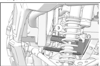
Install rear of winch mount with two carriage boltsand two nuts 4.
