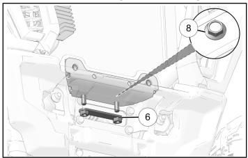
5. Install front of support bracket with two fasteners8 and two nuts 4.
