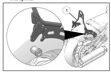
4. Close the backrest Lock & Ride® levers ® and install the retained safety screws (A). Torque to specification.
