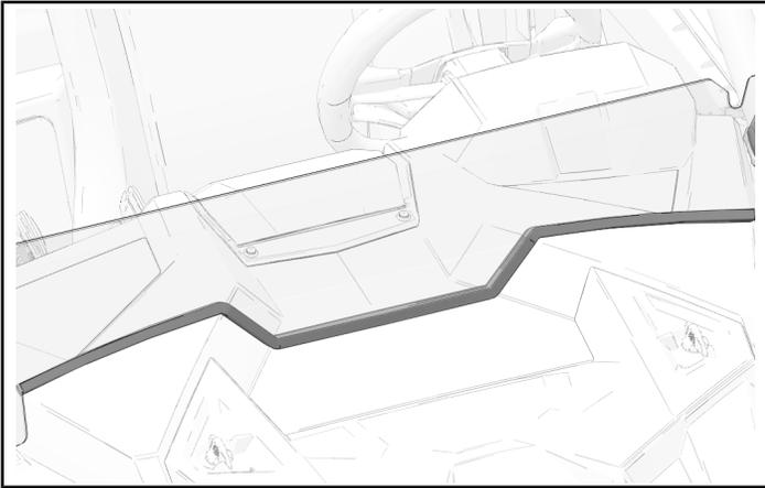
3. With windshield in correct position, attach to ROPS with two Lock & Ride® clamps.
