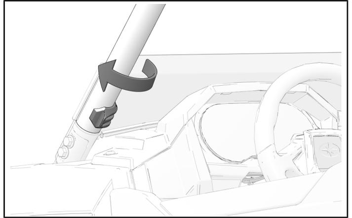
4. Windshield may need repositioning. If needed, release clamps and move windshield up along ROPS.
