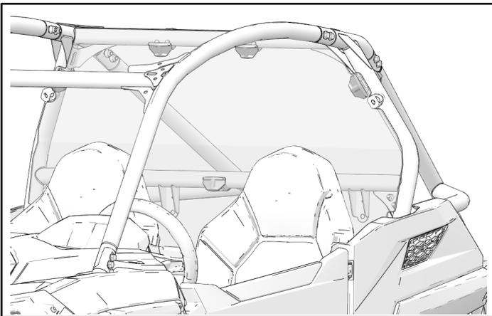
3. Move rear panel upwards until Lock & Ride® clamps are on horizontal tubes.
