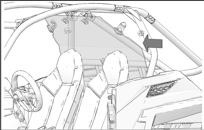
2. Align Lock & Ride® clamps with roll-cage tubes.
