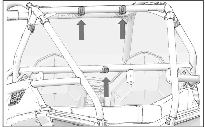
4. Apply pressure to outside of Lock & Ride® clamps to install onto roll-cage.
