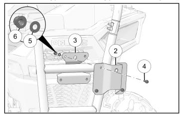
2. Pivot bracket assembly until the profile is parallel with the rear bumper's vertical tubes.
