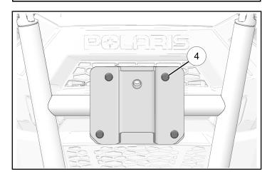
4. Align handle ① with bracket and turn clock-wise to install handle.
