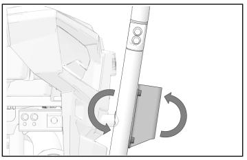
3. Counter-hold nuts and torque four bracket fasteners (4) to specification.
