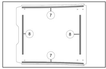
2. Install six U-nuts 6 onto roll-cage mounting plates.
