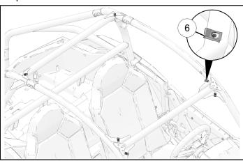
3. Install front of roof panel with two spacers ⑤ (between roof and U-nut), two washers ③, and two fasteners ④.
