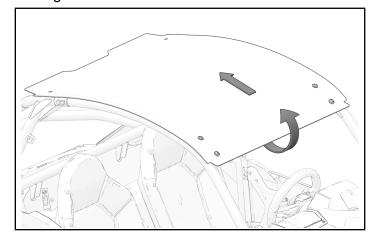
6. Install rear of roof with two washers ③ and two fasteners ②.
