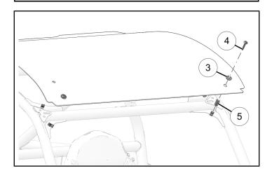
4. Install roof panel with two washers ③ and two fasteners ④. Torque four front fasteners ④ to specification.
