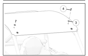
5. With front of roof secured to roll-cage, begin to slowly pull roof back so that it molds to the roll-cage's curvature.
