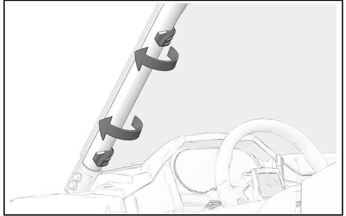
4. Windshield may need repositioning. If needed, release top clamps and slide windshield up along ROPS.
