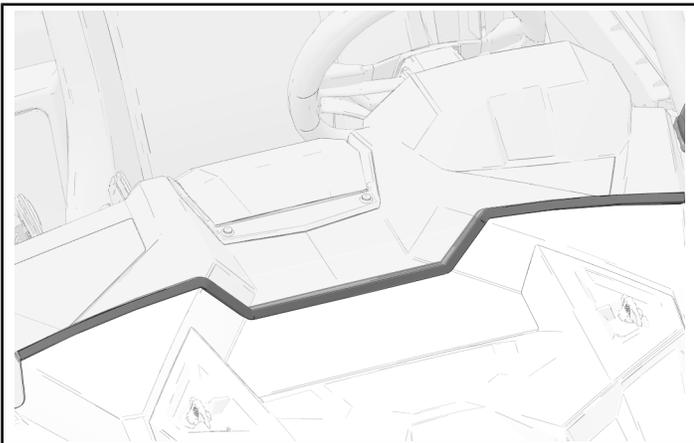
3. With windshield in correct position, secure to ROPS with four Lock & Ride® clamps.
