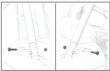
2. Insert accessory fastener ② and partially thread into accessory nut ④. Do not thread fastener past nut.
