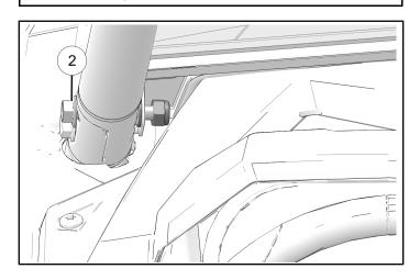
5. Continue to thread fastener ② through accessory nut and into lower mounting bracket. Begin to thread retained nut onto end of fastener ②.
