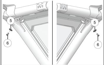
8. Tighten two retained nuts.
