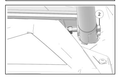
6. Torque two lower mounting fasteners ② to specification. Retained nuts will be tightened at a later time.
