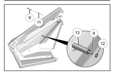
From inside inner door panel, insert one fastener
