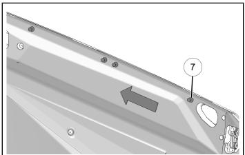
7. Beginning from front-most location, install seven push-pin rivets (3) (shorter).
