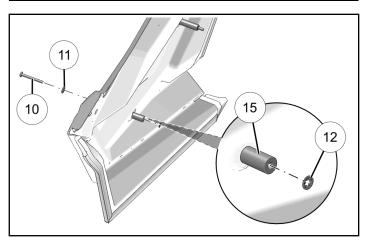
3. Remove and discard three fasteners holding plastic door panel to door frame.
