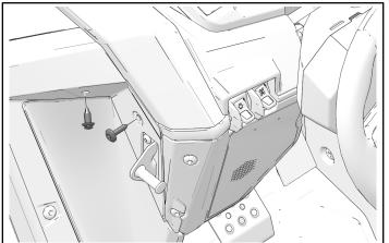
2. Slide door bracket ③ behind fender flare and install with retained push-pin rivet and one fastener.
