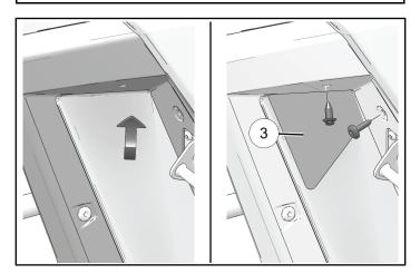
3. Torque fender flare fastener to specification.
