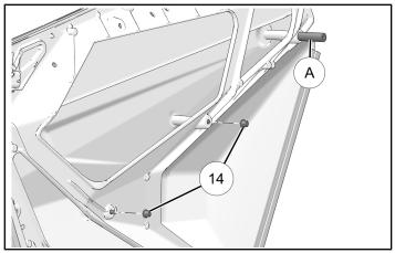
6. Counter-hold two nuts (14) and torque fasteners (9) and (10) to specification.
