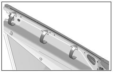
3. From outside of door, torque two shorter fasteners④ and four longer fasteners ③ to specification.
