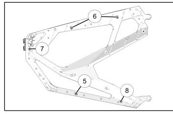
2. Install fastener and spacer combinations onto door casting. Make sure fasteners and spacers are centered on hole for best fitment. Spacer (6) and fastener (4) shown; others similar.
