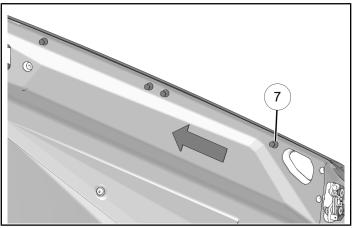
2. Beginning from front-most location, install seven push-pin rivets (8).
