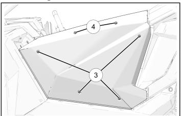
2. Make sure edge of inner door panel is under aluminum door panel.
