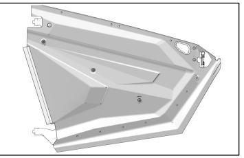
5. Install remaining spacer (A), from *Aluminum Door Kit*, onto rear most fastener. Install two nuts (A) (included with *Inner Door Kit*) on front-most fasteners.
