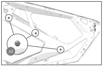
4. Align inner door panel with door frame and install inner door fasteners (9) and (10) to U-nuts in plastic door panel.
