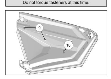
5. Make sure edge of inner door panel is under plastic door panel.
