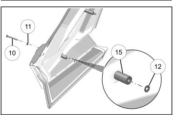
4. Align inner door panel with door frame.
