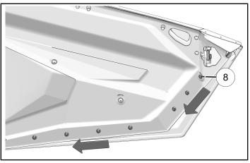
3. Make sure edge of inner door panel is under aluminum door panel.
