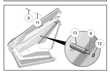
From inside inner door panel, insert one fastener
