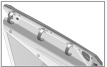
6. Beginning from front-most location, install four push-pin rivets ⑦ (longer).
