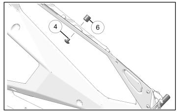
From inside of door, torque two shorter fasteners
