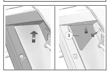
3. Torque fender flare fastener to specification.
