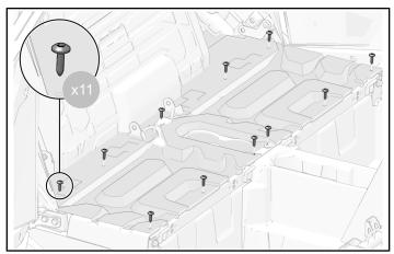
2. Reinstall one push-pin rivet in right-rear of seat panel.
