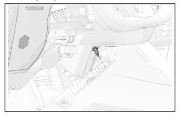
2. Install retained push-pin rivet and fuse block fastener. Torque two fuse block fasteners to specification.
