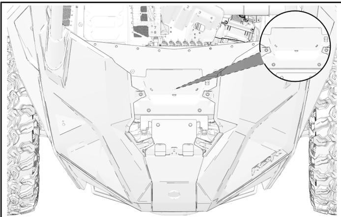
2. With a utility knife, carefully cut around edges of indentation.
