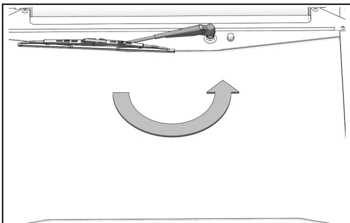
8. Secure wiper arm with washer ③ and nut ②.
