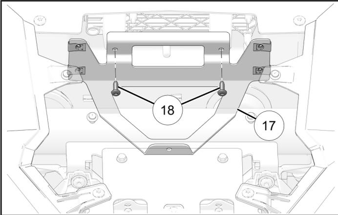
6. Install front of bottle mounting bracket ⑰ onto chassis with one fastener ⑱.
