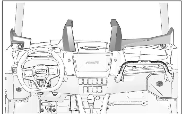
2. Open glove box lid. Remove and retain four dashboard fasteners around glove box opening.
