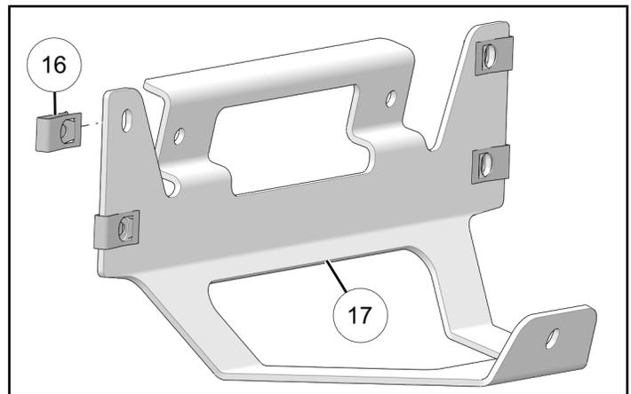
4. Install one U-clip nut ㉖ onto vehicle chassis.
