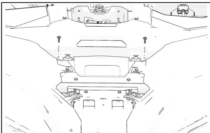
5. Install hood panels to with two retained push-pin rivets
