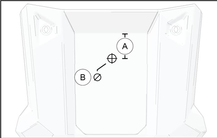
2. Pass nozzle **23** through hood panel and secure with nozzle nut.
