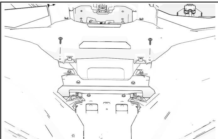
6. Remove and retain two push-pin rivets from front side hood panels.
