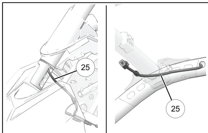
5. Secure ROPS harness to vehicle with edge clip ⑳.
