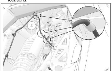
6. Route light bar harness ④ through grommet in firewall.
