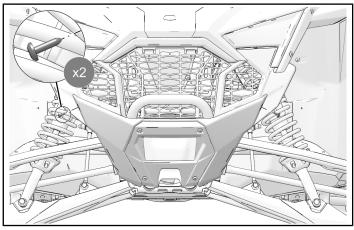
2. Install bottom front fascia with retained fasteners (shorter).
