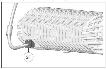
3. Place light bar onto mounts and torque two end nuts to specification.
