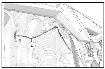
Reach through empty storage compartment and pull light bar harness from firewall grommet.
