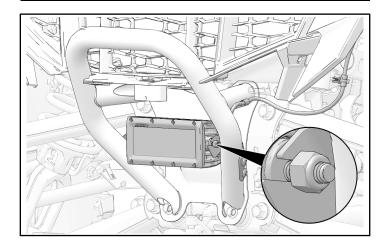
4. Install light bar harness ④ along vehicle structure and radiator shroud with edge clips.
