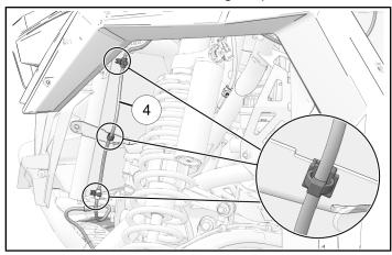
5. Route light bar harness ④ from driver side to passenger side. Attach harness to chassis electrical harness with cable ties ⑤ at taped locations.
