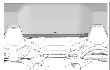
6. Press side clamps downward to engage on top of horizontal ROPS.
