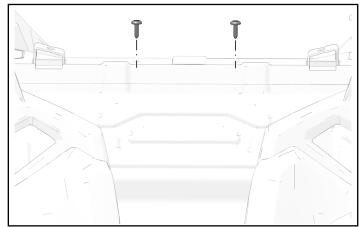
2. Install rear panel bracket ③ with two retained fasteners. Make sure vertical part of bracket is facing rearward.
