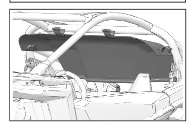
4. Carefully position rear panel so that side clamps rest on horizontal ROPS.
