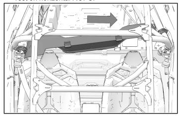
5. Compress seal to fit securely against body panel. Make sure mounting bracket is outside of rear panel.
