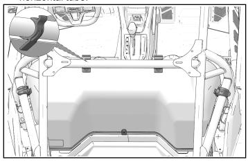
8. Secure rear panel to bracket with knob fastener ②.
