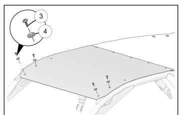
6. With front of roof panel secure to ROPS, begin to slowly pull roof panel back so that it molds to the curvature of the ROPS.
