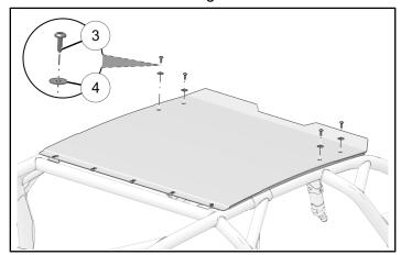
5. Install front roof panel ① with four fasteners ③ and four washers ④.
