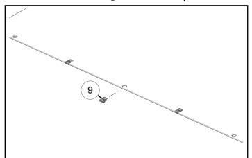
2. Install six U-nuts (9) onto middle and rear ROPS brackets.
