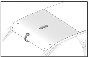
7. Install front roof panel to rear roof panel and middle ROPS brackets with five fasteners ③ and five washers ④.
