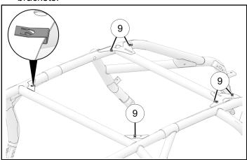
3. Install four U-nuts (9) onto front ROPS brackets.
