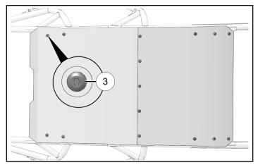
10. Torque rear roof fasteners to specification.
