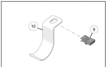
9. Install each tube hook bracket <sup>®</sup> with one fastener (3) and one washer (4).
