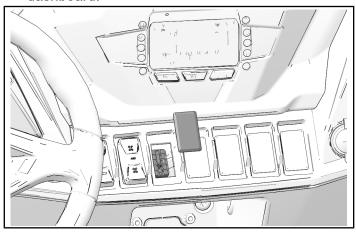
6. Slide connector **10F** through dashboard and align to switch (9).
