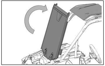
2. Lower roof into place and tighten bolts on top of windshield.
