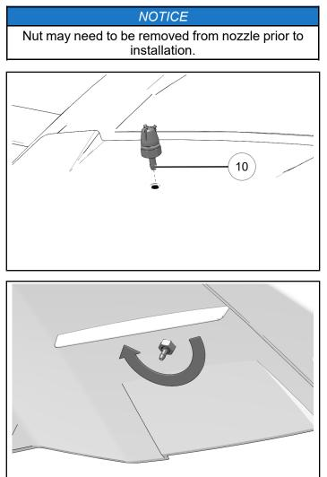
2. Connect wiper washer hose 2 to wiper nozzle 10.
