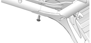
4. Remove locking screw from clamp on both left and right forward ROPS bars.
