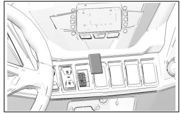
6. Slide connector **10F** through dashboard and align to switch **(9)**.
