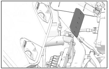
3. Remove one screw from each side as shown from roof.
