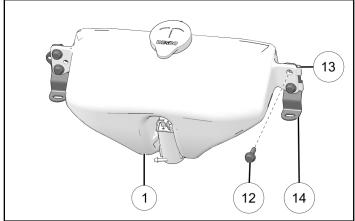
3. Install washer fluid hose (2) to the bottom of the washer fluid pump.
