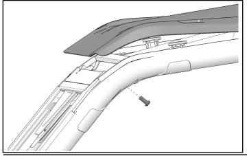
3. Attach side clamps on both left and right forward ROPS bars and use rubber mallet to secure it in place.
