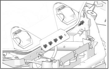
2. Remove retaining plate from windshield.
