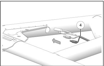
2. Pull ROPS wiper harness ④ from bottom of passenger-side ROPS frame and align connectors with main wiper harness connectors ①.
