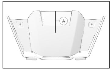
2. Drill 21/64 in (8.5 mm) hole in position marked on hood.
