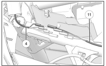
3. Connect ROPS wiper harness ④ to main wiper harness ① as shown.
