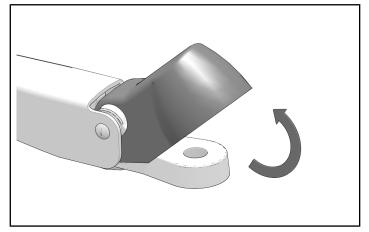
Install wiper arm onto wiper arm shaft with washer
