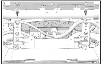
7. Install washer bottle assembly to chassis using two new screws (5).
