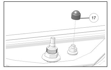
8. Lift wiper arm cap to reveal mounting bracket.
