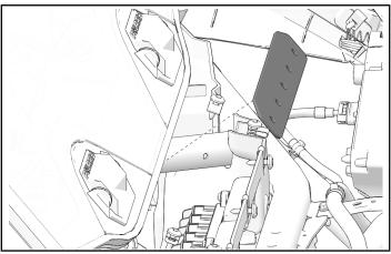
7. Attach push darts to retaining plate in windshield.
