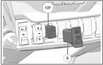
7. Connect switch (9) to harness connector **10F** and snap into place on dashboard.
