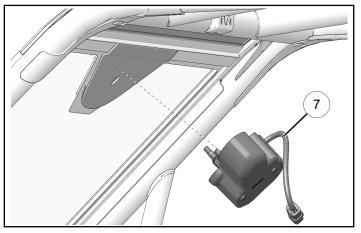
4. Attach motor to windshield frame with the following hardware:
