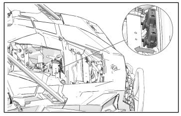
9. Remove cap from Polaris Pulse<sup>®</sup> bar and install power connector **1F**.
