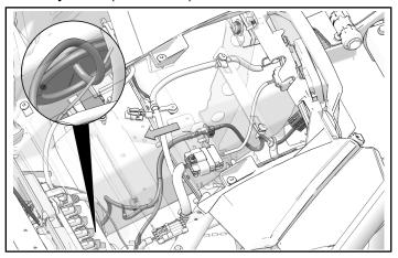
4. Place switch connector **10F** near switch plate.
