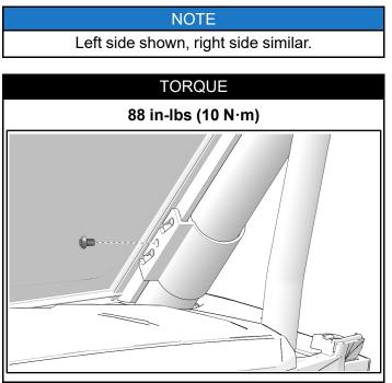
5. Attach two screws as shown to secure roof.
