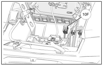
5. Remove and discard blank switch plate from dashboard.
