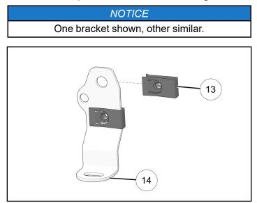
2. Install two brackets (4) to washer fluid bottle (1) with four speed nuts (13) and four screws (12).
