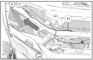
3. Route washer pump connector 2F through firewall grommet. Leave windshield switch (9) and fuse relays **10F** (not shown) for later connection.
