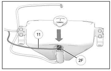
5. Attach clip tie ③ to mounting bracket ⑭, and route main wiring harness ⑪ and fluid hose ② through clip.
