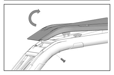
7. Lift front of roof and carefully tip windshiled out and clear it from vehicle. Store in a safe location.
