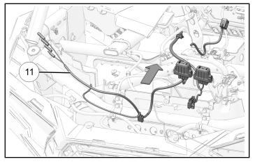
2. Route four bullet connectors of main harness (1) towards hole in the bottom of the passenger-side A-pillar.
