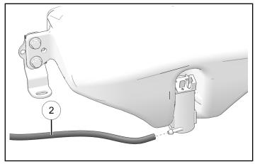
4. Connect main wiring harness (1) to washer fluid pump with connector **2F**.
