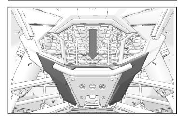
6. Reinstall top front fascia with kept fasteners (longer).
