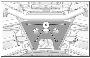
5. Reinstall front fascia panel to installed position.
