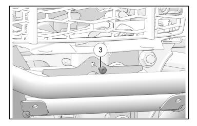
4. Install bumper plate to bumper with four plate fasteners (4).
