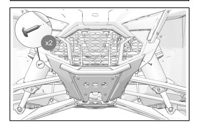
7. Reinstall bottom front fascia with kept fasteners (shorter).
