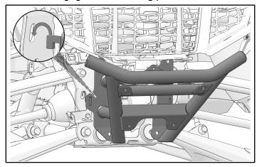
2. Install bumper to mounting plate with four bumper fasteners (5).
