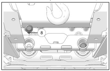
7. Torque bumper fasteners to specification.
