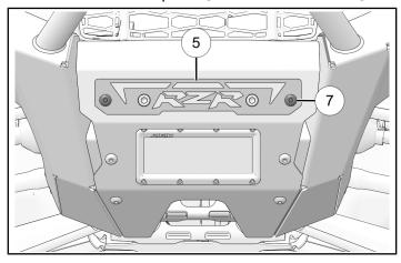
10. Torque bumper plate fasteners ① to specification.
