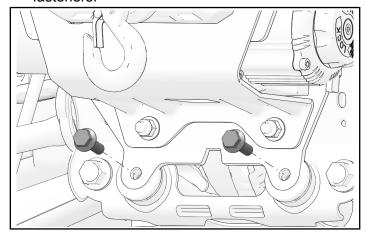
2. Remove and discard two fairlead fasteners.
