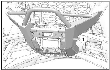
5. Install top of bumper with two fasteners 9.
