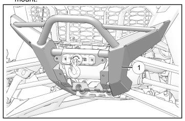
5. Put two fasteners (9) through fairlead and install top of bumper to winch mount.
