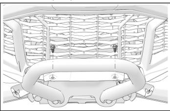
2. Remove four bumper fasteners to remove bumper assembly from chassis.
