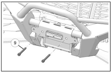
6. Install bottom of bumper with two fasteners **8**.
