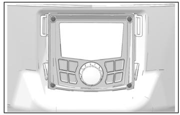
5. Install bezel to head unit bracket with two fasteners. Torque fasteners until fully seated.
