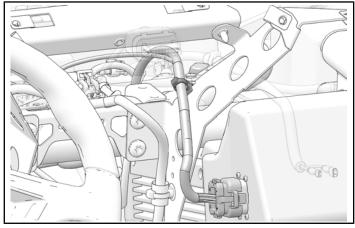
11. Install subwoofer connector **15M** to subwoofer.
