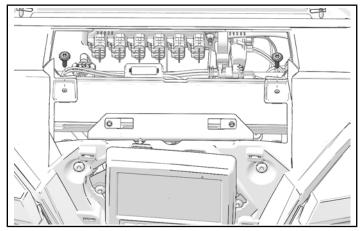
6. Remove and keep two lower bezel fasteners.
