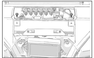
7. Torque four bezel fasteners to specification.
