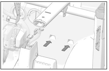
2. Drill two holes through dimples between indentations, identified in previous step.
