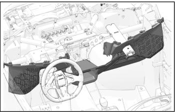
2. Install front dashboard with two fasteners.
