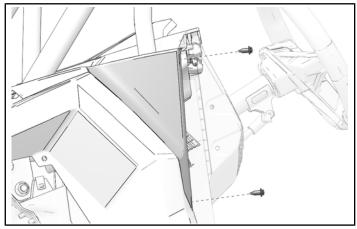
2. Rotate rear pocket fender away from vehicle body and remove.
