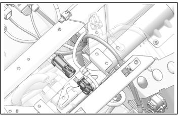
9. Install line-in connector 4M to audio harness.
