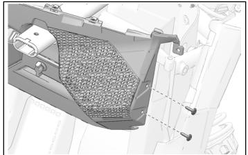
3. Remove and keep two fasteners from front dashboard.
