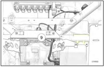
2. Install fuse relay to chassis tube, located to the right of the Polaris Pulse® bar.
