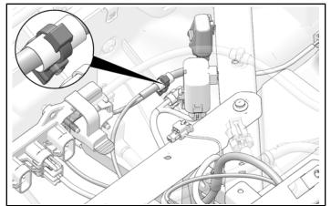
4. Remove and keep one nut from the negative terminal on the Polaris Pulse<sup>®</sup> bar.
