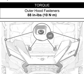
3. Place front pocket fender around ROPS bar and into outer hood slots.
