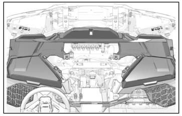
2. Install upper dashboard with five fasteners.
