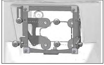
5. Remove one fastener to remove head unit bracket.
