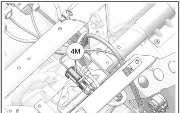
10. Install subwoofer harness under brackets, as shown, and connect to right-hand bracket with one edge clip.
