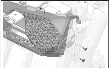
3. Install front dashboard with two fasteners.
