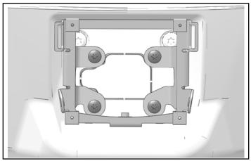
2. Install one fastener through hole and into U-nut. Torque fastener until fully seated.
