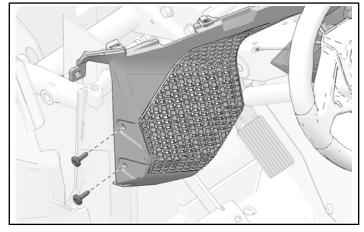
4. Remove two fasteners from front dashboard compartment.
