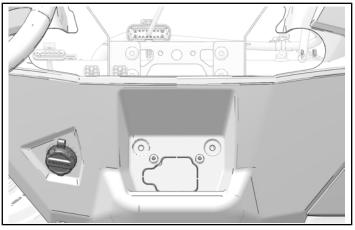
5. Ride Command<sup>®</sup> equipped vehicles only: Install front dashboard with two fasteners.
