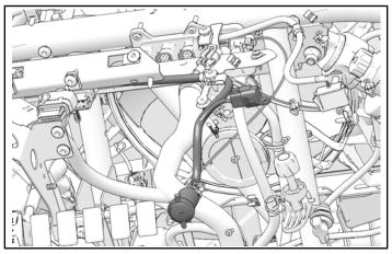
3. Make sure the ground wire does not get pressed between the subwoofer and speakers.
