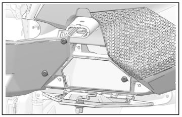
2. Remove and keep two fasteners from front dashboard.
