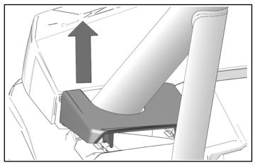
5. Remove and keep four outer hood fasteners.
