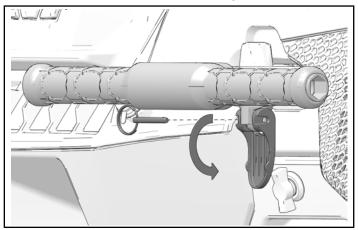
2. Remove top retaining pin to remove passenger handle.
