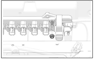
5. Install ground ring **1F** (black) to negative terminal with retained nut. Torque nut to specification.
