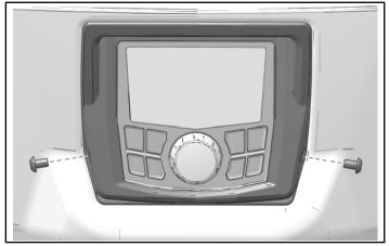
2. Remove four screws to disconnect PMX unit from mounting bracket.
