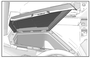
4. Remove and keep two storage compartment fasteners.
