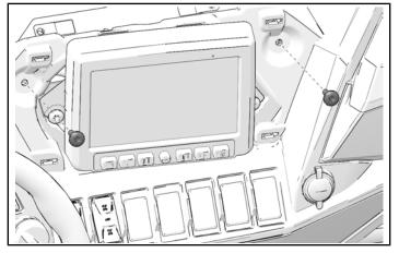
6. Install bezel with two upper fasteners.
