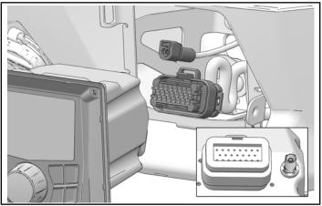
4. Install head unit to bracket with four retained fasteners. Torque fasteners until fully seated.
