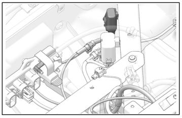
3. Attach the harness to a ridge on the front panel.
