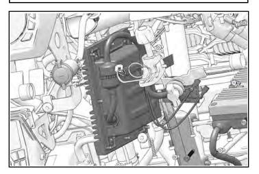
7. Install ground strap to chassis tube with one screw6. Torque screw until fully seated.
