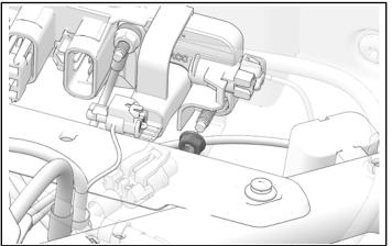
7. Install positive ring **1F** (red) to positive terminal with retained nut. Torque nut to specification.
