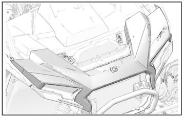
2. Install outer hood fasteners with four retained fasteners. Torque the four fasteners to specification.
