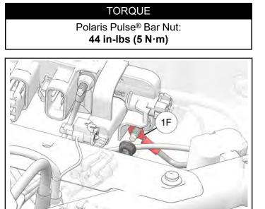
8. Remove and discard cap from subwoofer connector on PMX or Ride Command<sup>®</sup> harness.
