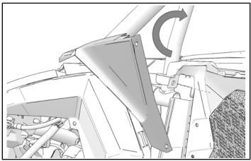
2. Attach rear pocket fender to vehicle using two push-pin rivets.
