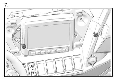
8. Carefully pull bezel away from dashboard. Reach behind bezel and disconnect all remaining electrical connections.
