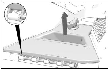
2. Align storage net ④ with front dashboard and pull three rubber ends through openings in dashboard.
