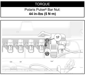
6. Remove and keep one nut from the positive terminal on the Polaris Pulse® bar.
