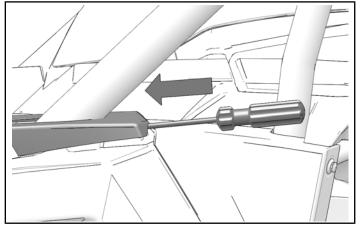
3. Gently lift screwdriver upward to free front pocket fender from clips.
