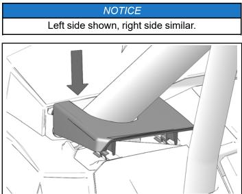
4. Gently push tab into clips until front pocket fender is secure.
