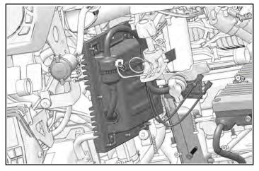
4. Tilt subwoofer upwards and hook clamps over chassis cross-beam, as shown. Torque clamp fasteners to specification.
