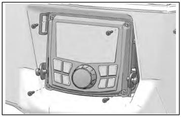
3. Pull PMX head unit out and disconnect antenna and power connectors.
