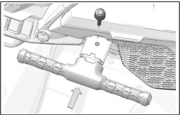
2. Align lever with top retaining pin and install side retaining pin.
