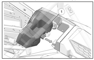
3. Install the speaker to the vehicle with two fasteners ③. Torque fasteners until fully seated.
