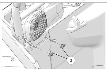
4. Identify the chassis harness speaker connector in the wheel well.
