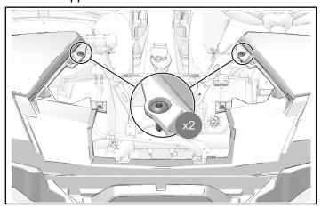
4. Torque the seven dashboard fasteners to specification.
