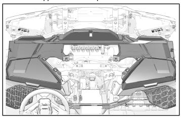
2. Install upper dashboard with five fasteners.
