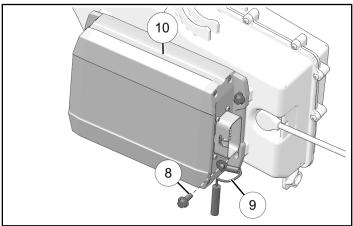
Put speaker into installed position with clamp installed around chassis tube. Make sure speaker harness is not pinched between speaker and vehicle.
