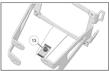
5. Install head unit bracket to front dashboard compartment with four screws ①. Torque screws until fully seated.
