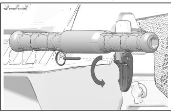
2. Remove top retaining pin to remove passenger handle.
