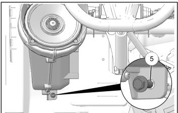
2. Install module and connector to chassis with attached push-darts.
