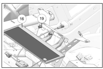
4. Install antenna connector to audio harness.
