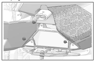
7. Torque the dashboard fasteners to specification.
