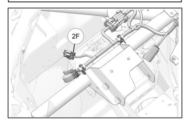
10. Put head unit connector **23F** between support brackets and install to right-hand bracket with push-pin clip, as shown.
