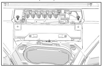
6. Remove and keep two lower bezel fasteners.
