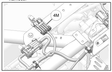
8. Install audio harness to vehicle with edge clips, as shown.
