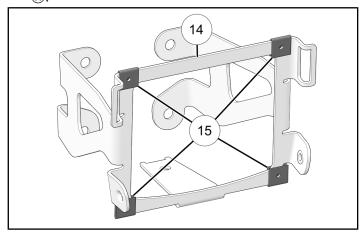
4. Install one large U-nut <sup>®</sup> onto bottom of head unit bracket.
