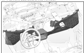
2. Install front dashboard with two fasteners.
