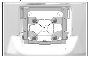
6. Install one screw <sup>(9)</sup> through drilled hole and into U-nut. Torque screw until fully seated.
