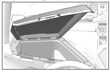
4. Remove and keep two storage compartment fasteners.
