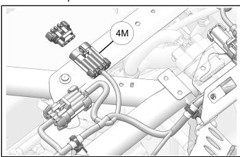
6. Rear audio equipped vehicles only: Remove cap from rear audio connector on main vehicle harness.
