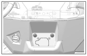
6. Open glove box and install three fasteners.
