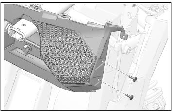
3. Install front dashboard with two fasteners.
