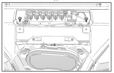
7. Torque four bezel fasteners to specification.
