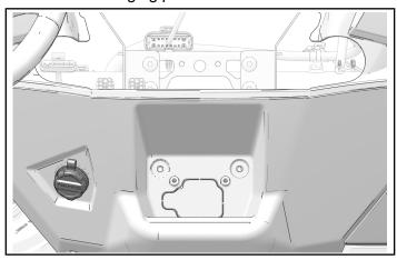
5. Install front dashboard with two fasteners.
