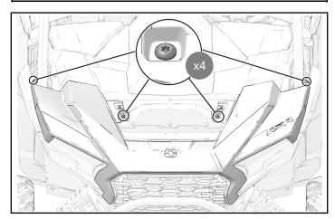
3. Place front pocket fender around ROPS bar and into outer hood slots.
