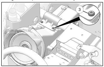
3. Install ground ring to chassis tube with screw 19.
