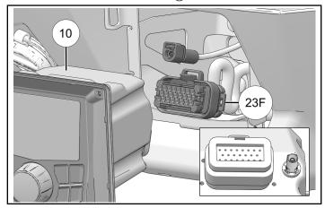
2. Install head unit (10) to bracket with four screws (12). Torque screws until fully seated.
