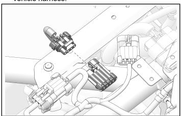
Rear audio equipped vehicles only: Install rear audio connector 4M to main vehicle harness.
