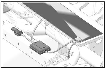
7. Tighten clamp fasteners 3 until fully seated.
