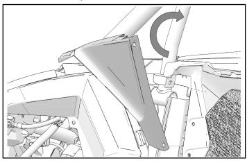
2. Attach rear pocket fender to vehicle using two push-pin rivets.
