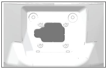
2. Identify "X" on bottom of front dashboard and drill one **1/4 in 6 mm** hole in the center.
