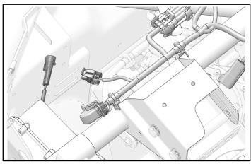
Stage 2 Audio Kit Only: Install amp and ground connectors to amplifier.
