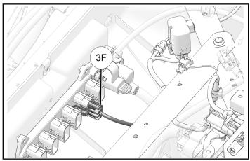
3. Install fuse relay to chassis tube.
