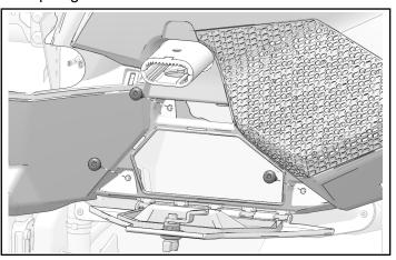
2. Remove and keep two fasteners from front dashboard.
