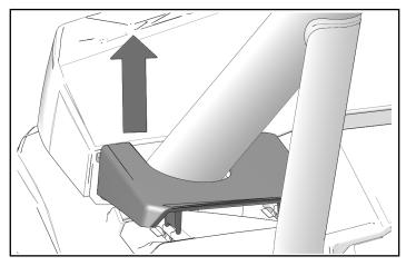
5. Remove and keep four outer hood fasteners.
