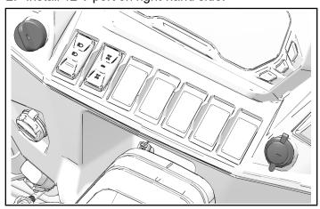
3. Push bezel into dashboard so that clips engage with dashboard.
