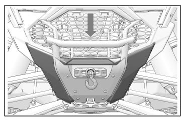
10. Reinstall top front fascia with kept fasteners (longer).
