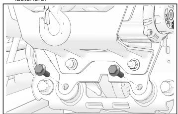
2. Remove and discard two fairlead fasteners.
