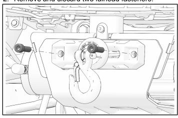
3. Turn winch lock to "FREE" to pull out winch cable. Put winch hook and fairlead through opening in bumper.
