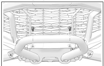
2. Remove four bumper fasteners to remove bumper assembly from chassis.
