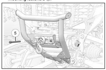
6. Install front bumper with two bottom mounting fasteners 4.
