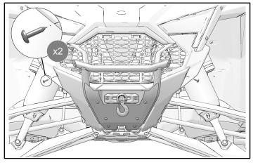
11. Reinstall bottom front fascia with kept fasteners (shorter).
