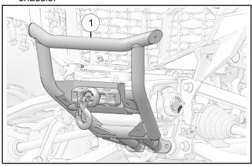
5. Install front bumper and fairlead with two top mounting fasteners ⑤.
