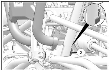
6. With bumper properly aligned, torque four fasteners to specification.
