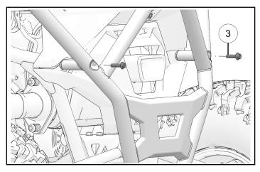
4. Pass two bottom mounting fasteners ④ through bumper mounts and transmission mount to ensure alignment.
