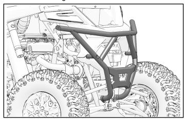
3. Secure bumper to top-rear fascia and chassis with two top mounting fasteners ③.
