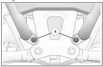
5. Wrap one plate nut ② around each vertical tubes. Thread each fastener into plate nut.
