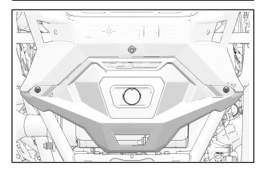
2. With an assistant, align bumper with vehicle rear. Align top mounting arms with top-rear fascia and lower mounting arms with transmission mount.
