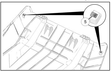
5. Clean seal channel on rear roof panel 2 with isopropyl alcohol.
