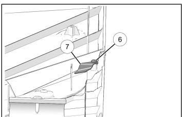
11. Put roof panel on top of roll-cage.
