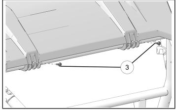
16. Torque two roof fasteners 4 to specification.
