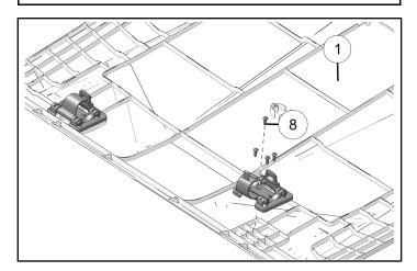
3. Install seal <sup>®</sup> onto front of panel, as shown.
