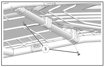
15. Install rear roof panel to roll cage with two fasteners ③. Torque fasteners to specification.
