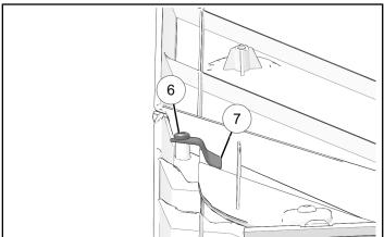
10. Install right corner roof bracket **(6)** with one screw **(7)** and torque fastener until fully seated.
