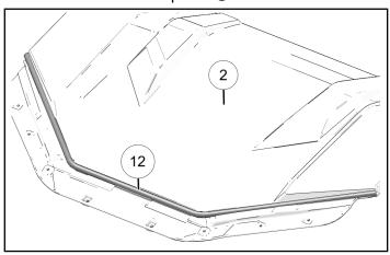
7. With both roof panels upside down, align rear roof panel with bosses on front roof panel.
