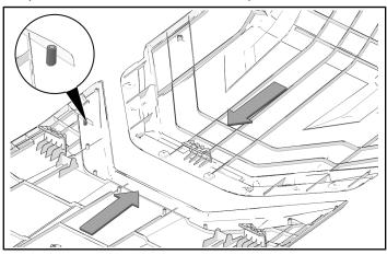
8. Install roof panels together with eight screws (8). Torque fasteners until fully seated.
