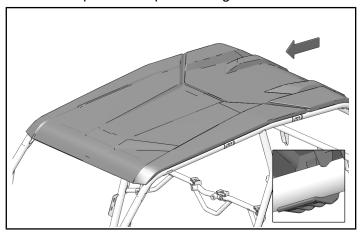
12. Install roof panel to roll cage with two fasteners 4 installing into U-nuts (5) (previously installed).
