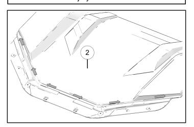
6. Peel paper backing from seal @ and install seal in channel of rear roof panel 2.
