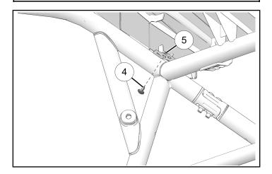
13. Install roof panel to roll cage with two clamp assemblies.
