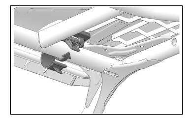
14. Install rear roof panel to center tube with two fasteners 3. Torque fasteners to specification.
